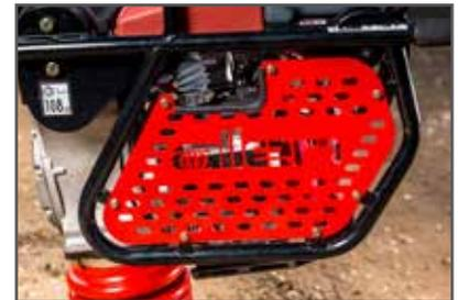
Steel protective gaurds prevent damage to key engine components.
