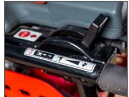
The multi-functional level controls the throttle, fuel supply and shut off.
