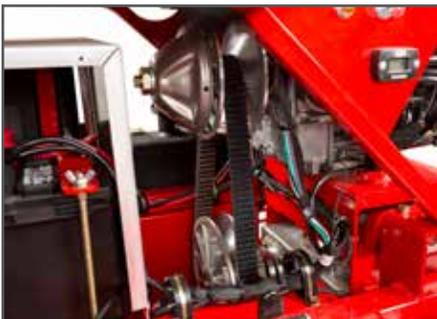
Specially tuned torque converter clutches provide excellent low end torque and superior high rotor speed for burnishing concrete.
