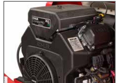
Two Kohler EFI 26.5 hp gasoline engines provide maximum power output to the rotors through electronic fuel injection.
